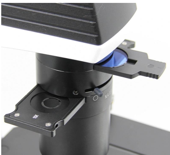
Filters: Blue, Dia.34mm; Green, Dia.34mm
